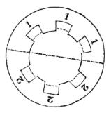
the grooves are made of the same width at the bottom and top, as shown at 2, 2, 2, which is, for grooves of the depth of which they are made, practically the same, as the dotted circle will show. Our gun-makers use from six to ten grooves.
