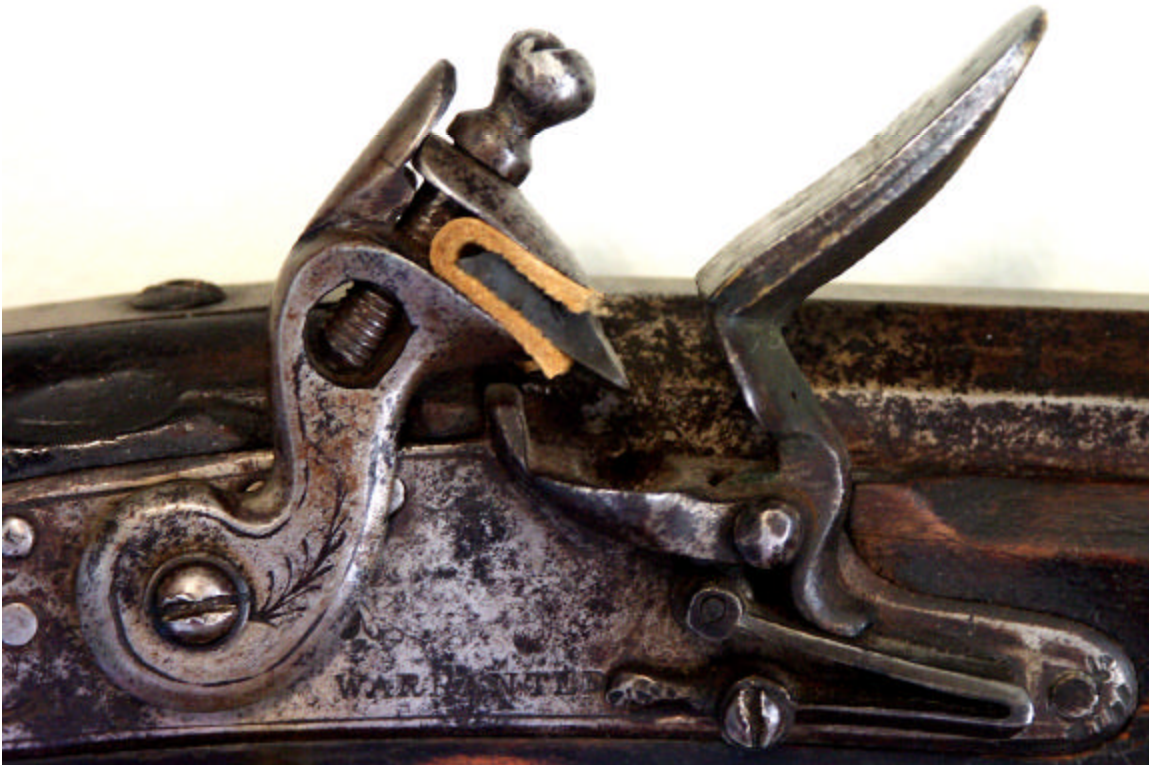
American flintlock rifle, late style, with a piece of steel nearly 1/16” (1.5mm) thick brazed onto the frizzen. The rifle itself shows very little signs of use, so this was might have been done when the lock was made. Capt. John G.W. Dillin illustrates this rifle, from the Clarence St John collection, as No. 3, Plates 93 & 94.
